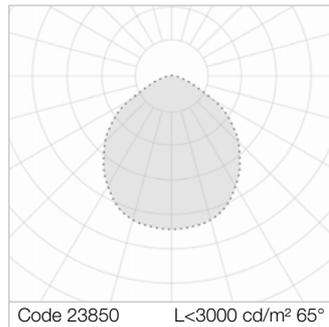
Average luminance <math><3000\text{ cd/m}^2</math> for angles >math>65^\circ</math>. Installation Interdistance Transv.D = 1.20 x hu - Long.D = 1.20 x hu. Rhomboidal lenses with differentiated surfaces, etched and prismatic to optimise the orientation of the luminous flux, in opal methacrylate (PMMA).
