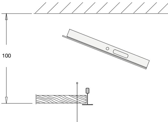
Installation following false ceiling mounting, supported by the exposed structure, minimum void of 110 mm from the structure's lower edge.
