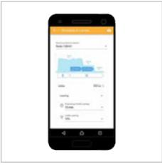
Free app for configuration of ZQ devices, available for Apple (iOS) and Android smartphones and tablets. Light360|Setup allows the installation to be split into groups of luminaires and sensors and to set control logics and operating parameters (reference light levels for constant light control, timeout for motion sensor power-off, etc.).
