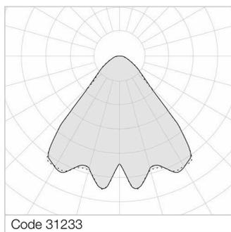
Wide lens in transparent methacrylate (PMMA).
