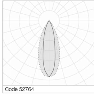
Symmetrical elliptical hyperconcentrated distribution. Polycarbonate screen etched internally, V2 self-extinguishing, UV stabilised, injection moulded.
