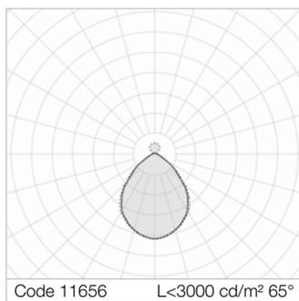
Average luminance <math><3000 \text{ cd/m}^2</math> for radial angles >math>65^\circ</math>. Light emission: direct 85%, indirect 15% . Flow recuperator in semi-glossy aluminium. LGS micro-prismatic flat diffuser in transparent methacrylate (PMMA), multi-lenticular exterior, anti-glare. Anti-glare opal polycarbonate filter for brightness uniformity. On request, indirect emission versions enhanced.
