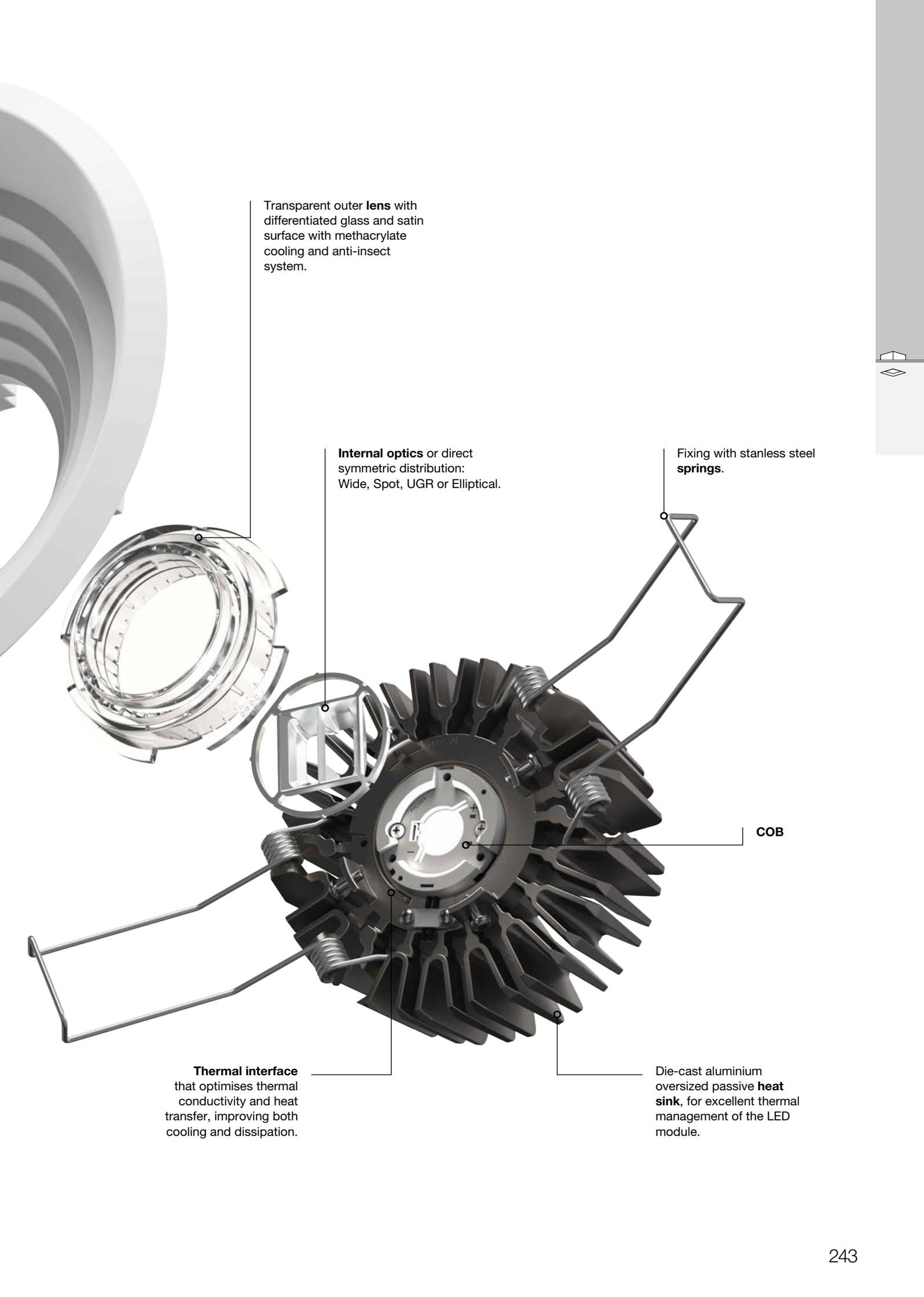
Transparent outer **lens** with differentiated glass and satin surface with methacrylate cooling and anti-insect system.
