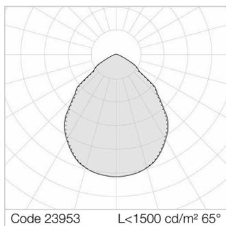
Average luminance <math>< 1500 \text{ cd/m}^2</math> for radial angles >65°. LGS micro-prismatic flat diffuser in transparent methacrylate (PMMA), multi-lenticular exterior, anti-glare. Anti-glare opal polycarbonate filter for brightness uniformity.
