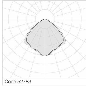
Wide symmetric lighting distribution. Polycarbonate screen etched internally, V2 self-extinguishing, UV stabilised, injection moulded.
