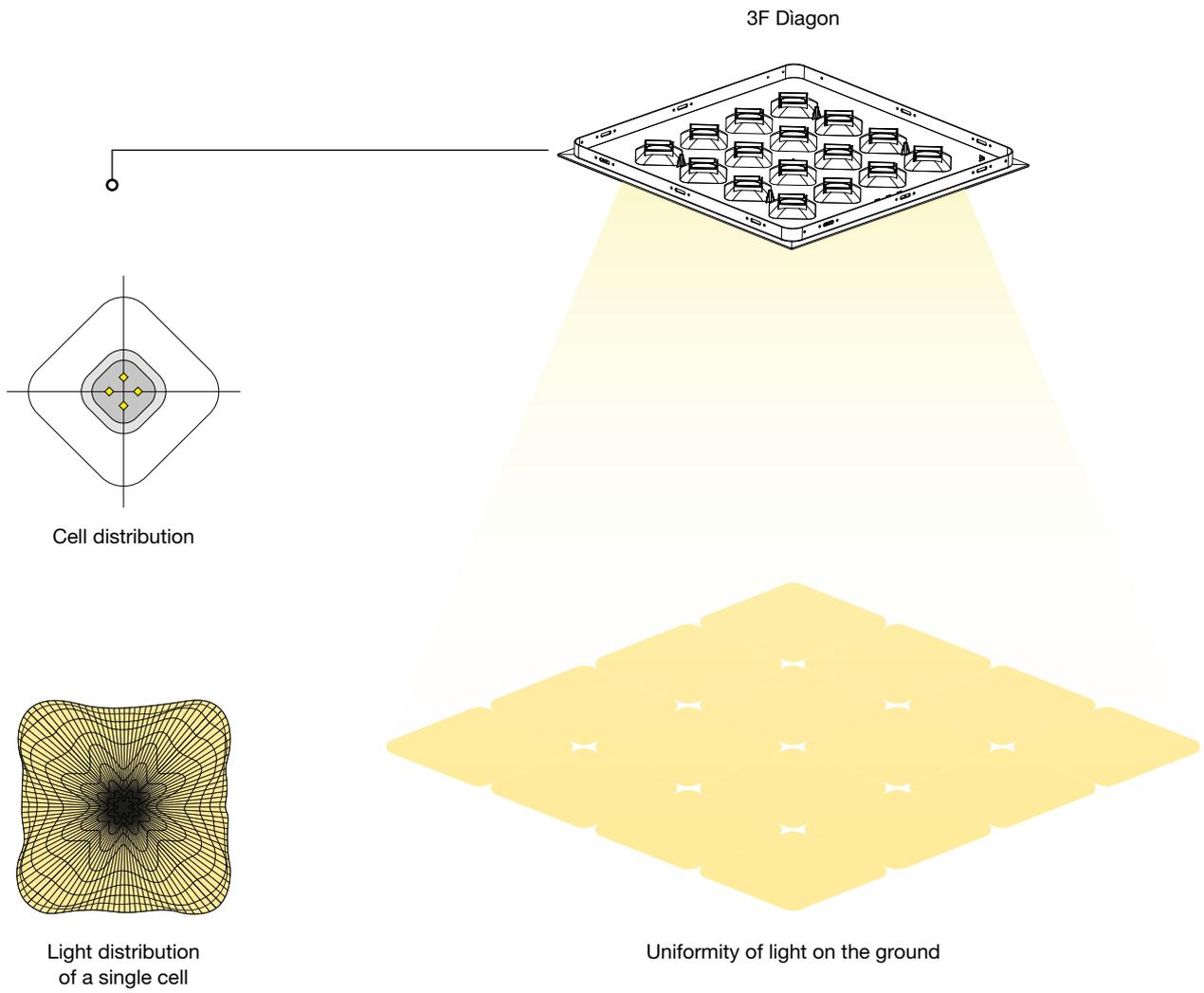
With this cells oriented at 45°, the uniformity on the ground is greater because the light distribution of the cell fills the space more.
