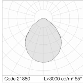
Average luminance <math><3000 \text{ cd/m}^2</math> for radial angles >math>65^\circ</math>. VSS moulded laminated dipped glass, non-combustible, thickness 7 mm. Anti-glare opal polycarbonate filter for brightness uniformity.
