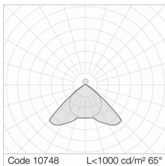
Average luminance <math><1000\text{ cd/m}^2</math> for radial angles >math>65^\circ</math>. Light emission: direct 85%, indirect 15% . 2MG parabolic louvre, high efficiency, in specular aluminium with superficial titanium-magnesium treatment, non-iridescent, with transverse blades closed at the top. Prismatic methacrylate (PMMA) diffuser for total shielding of the louvre compartment. Film protective against dust and finger marks, adhesive, attached to louvre.
