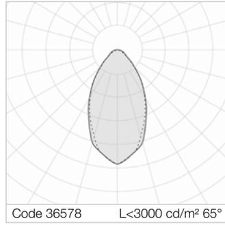
Average luminance <3000 cd/m<sup>2</sup> for radial angles >65°. VS moulded glass, anti-glare, tempered, non-combustible, thickness 4 mm.
