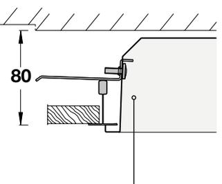
Minimum void of 80 mm from the structure's lower edge.
