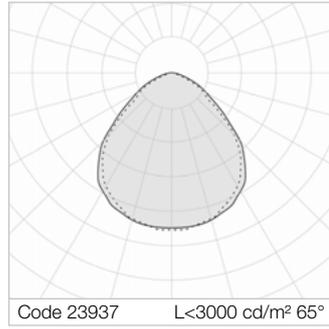
Average luminance <math><3000\text{ cd/m}^2</math> for radial angles >math>65^\circ</math>. SP transparent methacrylate (PMMA) diffuser, prismatic outside, antiglare.
