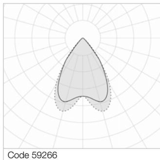
Medium distribution with square shape. Integrated DALI light and presence sensor on the luminaire, to keep lighting levels constant in accordance with the amount of natural light and the presence of persons. Turns on and off and is regulated according to the level of light and the presence of persons.
