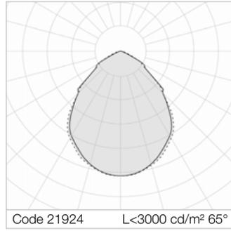
Average luminance <math><3000\text{ cd/m}^2</math> for radial angles >math>65^\circ</math>. SP transparent methacrylate (PMMA) diffuser, prismatic outside, antiglare. Anti-glare opal polycarbonate filter for brightness uniformity.
