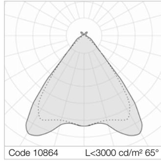
Average luminance <math><3000 \text{ cd/m}^2</math> for radial angles >math>65^\circ</math>. Transparent methacrylate (PMMA) controlled distribution lenses with flat external surface.
