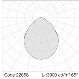
Average luminance <3000 cd/m² for radial angles >65°. VS moulded glass, anti-glare, tempered, non-combustible, thickness 4 mm. Anti-glare opal polycarbonate filter for brightness uniformity.
