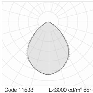
Average luminance <math>< 3000 \text{ cd/m}^2</math> for radial angles >math>65^\circ</math>. Flow recuperator in semi-specular aluminium, high efficiency. LGS micro-prismatic flat diffuser in transparent methacrylate (PMMA), multi-lenticular exterior, anti-glare. Anti-glare opal polycarbonate filter for brightness uniformity.
