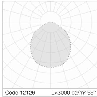
Installation Interdistance Transv.D = 1.20 x hu - Long.D = 1.20 x hu.
