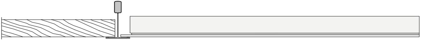
Panels in mineral fibre with exposed structure 600x600 or 625x625.
