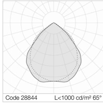
Average luminance <math>< 1000 \text{ cd/m}^2</math> for radial angles >math>65^\circ</math>. 2MG parabolic louvre, high efficiency, in specular aluminium with superficial titanium-magnesium treatment, non-iridescent, with transverse blades closed at the top. Prismatic methacrylate (PMMA) diffuser for total shielding of the louvre compartment. Film protective against dust and finger marks, adhesive, attached to louvre.
