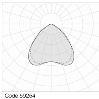
Wide distribution with rectangular shape. Integrated DALI light and presence sensor on the luminaire, to keep lighting levels constant in accordance with the amount of natural light and the presence of persons. Turns on and off and is regulated according to the level of light and the presence of persons.
