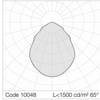
Average luminance <1500 cd/m<sup>2</sup> for radial angles >65°. LGS micro-prismatic flat diffuser in transparent methacrylate (PMMA), multi-lenticular exterior, anti-glare, locked to the white painted aluminium perimeter frame, hinged opening. Anti-glare opal polycarbonate filter for brightness uniformity.
