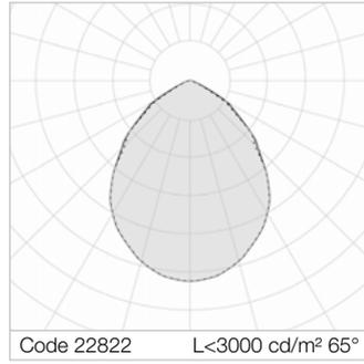
Average luminance <math><3000\text{ cd/m}^2</math> for radial angles >math>65^\circ</math>. LGS micro-prismatic flat diffuser in transparent methacrylate (PMMA), multi-lenticular exterior, anti-glare. Anti-glare opal polycarbonate filter for brightness uniformity.
