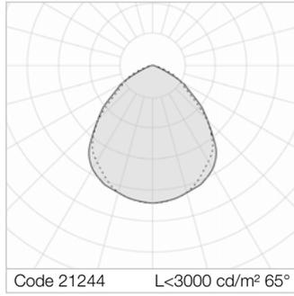
Average luminance <math><3000\text{ cd/m}^2</math> for radial angles >math>65^\circ</math>. SP transparent methacrylate (PMMA) diffuser, prismatic exterior, anti-glare, locked to the prepainted white aluminium perimeter frame with sealing gasket, hinged opening.
