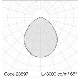
Average luminance <math><3000\text{ cd/m}^2</math> for radial angles >math>65^\circ</math>. VS moulded glass, anti-glare, tempered, non-combustible, thickness 4 mm.
