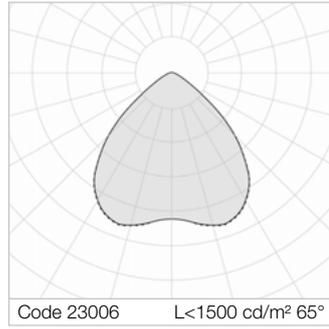
Average luminance <math><1500 \text{ cd/m}^2</math> for radial angles >math>65^\circ</math>. 39W - Average luminance <math><3000 \text{ cd/m}^2</math> for radial angles >math>65^\circ</math>. Installation Interdistance Transv.D = 1.40 x hu - Long.D = 1.40 x hu. Rhomboidal lenses with differentiated surfaces, etched and prismatic to optimise the orientation of the luminous flux, in transparent methacrylate (PMMA).
