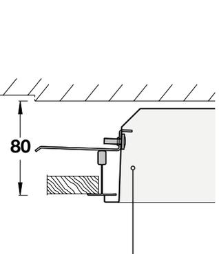
Minimum void of 80 mm from the structure's lower edge.
