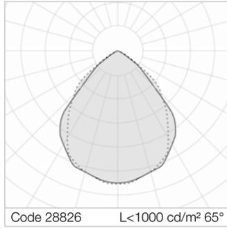
Average luminance <math><1000 \text{ cd/m}^2</math> for radial angles >math>65^\circ</math>. 2S parabolic louvre in semi-specular aluminium, non-reflecting, with transverse blades closed at the top. Prismatic methacrylate (PMMA) diffuser for total shielding of the louvre compartment. Film protective against dust and finger marks, adhesive, attached to louvre.
