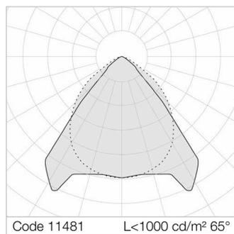
Average luminance <math><1000\text{ cd/m}^2</math> for radial angles >65°. 2MG parabolic louvre, high efficiency, in specular aluminium with superficial titanium-magnesium treatment, non-iridescent, with transverse blades closed at the top. Prismatic methacrylate (PMMA) diffuser for total shielding of the louvre compartment. Film protective against dust and finger marks, adhesive, attached to louvre.
