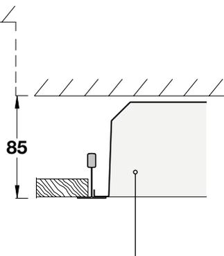
Installation simultaneously with the false ceiling, minimum void of 85 mm from the structure's lower edge.
