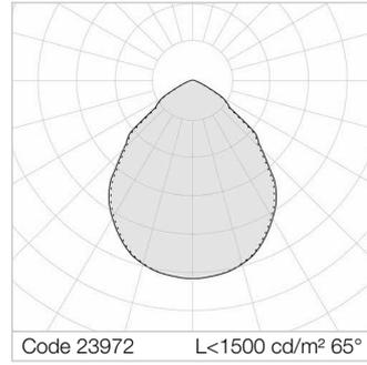
Average luminance <math><1500 \text{ cd/m}^2</math> for radial angles >math>65^\circ</math>. LGS micro-prismatic flat diffuser in transparent methacrylate (PMMA), multi-lenticular exterior, anti-glare. Anti-glare opal polycarbonate filter for brightness uniformity.
