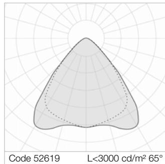
Controlled symmetric distribution. Average luminance <math><3000 \text{ cd/m}^2</math> for radial angles >math>65^\circ</math>. Polycarbonate screen etched internally, V2 self-extinguishing, UV stabilised, injection moulded.
