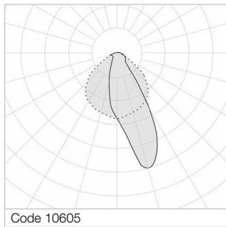
Transparent methacrylate (PMMA) asymmetric distribution lenses with a flat external surface.
