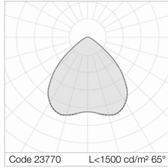
Average luminance <math><1500\text{ cd/m}^2</math> for radial angles >math>65^\circ</math>. Installation Interdistance Transv.D = 1.40 x hu - Long.D = 1.40 x hu. Rhomboidal lenses with differentiated surfaces, etched and prismatic to optimise the orientation of the luminous flux, in transparent methacrylate (PMMA).
