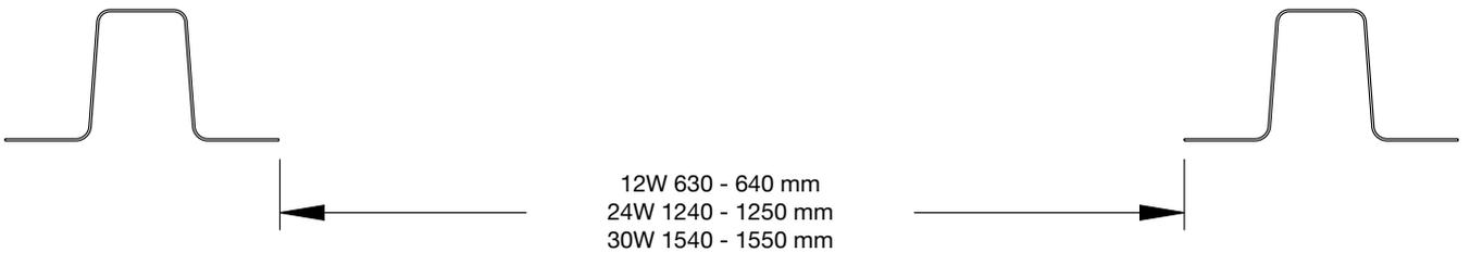
For perfect installation of the luminaires, the load-bearing profile sections should be positioned at the distances indicated above (net space between profiles).
